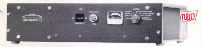
This new crystal oscillator combines high stability with the physical ruggedness necessary to withstand vibration and shock. It uses a 5-Mc, 5th-overtone crystal in an all-solid-state circuit of silicon transistors. Both crystal and circuit are held at constant temperature by a proportionally controlled oven. Fiberglas-epoxy etched circuits, cased transformers, and Mil grade electrolytic capacitors make the unit acceptable for many military and government applications.
