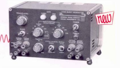
The Tone-Burst Generator is a unique instrument, which, when fed from an external oscillator, generates pulses, or bursts, of the input frequency. It is useful for testing the time response of ac circuits and for simulating the pulsed ac signals commonly used in audio and ultrasonic equipment, such as sonar.
